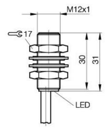
Inductive Sensors BES 516-329-E4-C-03 M12x1 x 33 normally-open Sn=2mm shielded
